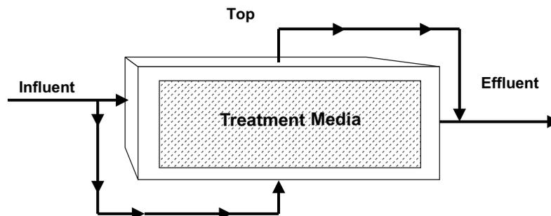
VSBs, as shown in figure 2, usually follow a septic tank and remove most of the suspended and larger colloidal particles, BOD, organic forms of nitrogen, and other particles. Although they are frequently identified as subsurface constructed wetlands, they do not fit the strict definition of a constructed wetland.
