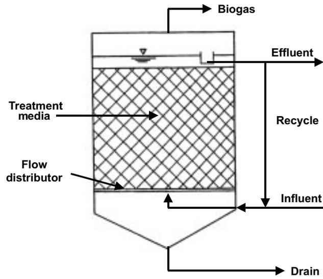
Figure 4. Schematic of the upflow anaerobic sludge blanket process
