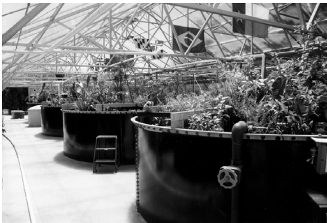
FIGURE 1 THE OPEN AEROBIC TANKS OF THE LIVING MACHINE® IN SOUTH BURLINGTON, VT
